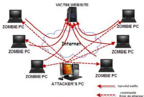
Figure 3. DDoS attack working model
